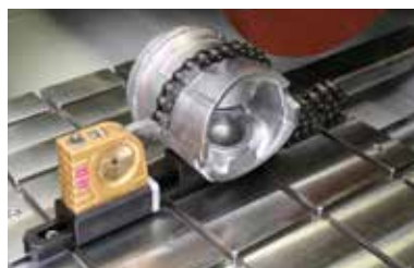
Guide bar with chain clamping vice
