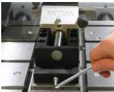
Change of preassembled Easy-clamping bases
