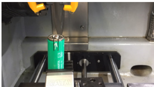
Sectioning of a complete LIB with QATM cut-off machine
