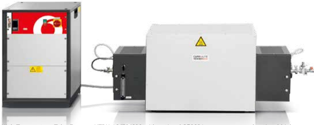
Horizontal High Temperature Tube Furnace HTRH 18/70/600 with optional 3508P1 programmer and optional high vacuum capable inert gas package (high vacuum capable up to 1450°C and up to 1800°C under normal pressure. Rotary vane pumps and turbo pumps optional available (see page 118).
